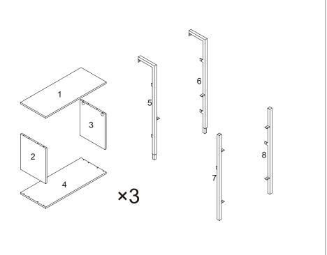
Attach piece 2 & 3 to piece 4 using wooden dowels (F), screws (C).
